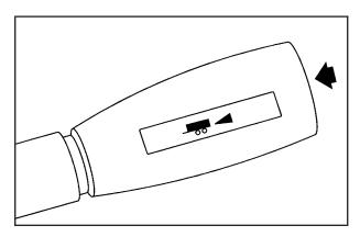
Press the button at the end of the shift lever to enable/disable the tow/haul mode.
